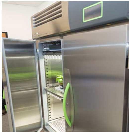
Plant Growth Chamber
