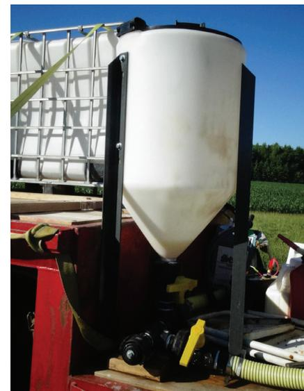
These inductors and vats are commonly used for mixing pesticides. Do not put more than one product in these mixing containers at a time. The risk of incompatibility is greater when you use low water volumes and high rates of crop protection products. Having more water in the tank decreases the chance of problems occurring.
